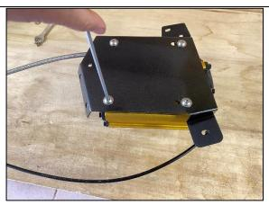
**STEP 1.7** ATTACH THE TANK TO THE JBA BRACKET USING M8 X 20 PAN HEAD WITH A WASHER UNDER THE HEAD AS SHOWN. FASTEN FROM UNDERNEATH USING M8 NYLOC AND WASHER.
