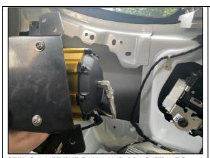
**STEP 2.1** LIFT THE TANK AND BRACKET INTO VEHICLE AND CONNECT THE JBA-CB111 400MM HOSE FROM THE COMPRESSOR AS SHOWN.
