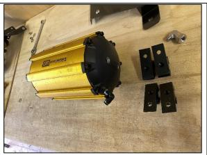
**STEP 1.2** IF FITTING OPTIONAL JBA TANK DRAIN KIT, FIT THE 90 DEGREE QUICK FIT ELBOW TO THE BOTTOM GRUB SCREW AS SHOWN.
