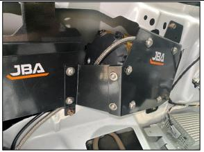
**STEP 2.4** FIX THE JOINER BRACKET USING M6 X 20 SCREWS WITH SPLIT WASHER THEN FLAT WASHER AS SHOWN. FULLY TIGHTEN ALL FASTENERS AT THIS POINT.
