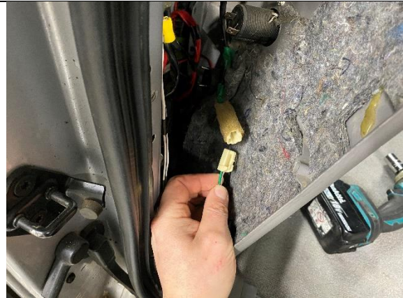
STEP 1.8 UNCLIP WIRING LOOM AS SHOWN
