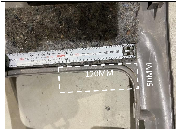
STEP 1.11 MARK FROM THE REAR OF THE QUARTER PANEL OPENING 120MM X 50MM AS SHOWN.
