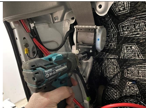
STEP 1.10 UNDO 14MM BOLT ON REAR SEAT BELT AND SET ASIDE.
