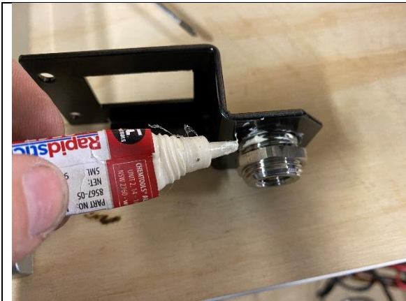
STEP 2A.1 INSTALL JBA-CB103 BULK HEAD TO THE SWITCH PLATE.
