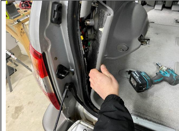
STEP 1.7 START PULLING BACK THE QUARTER PANEL FROM THE REAR DOOR AND THE ALONG THE BOTTOM OF THE WINDOW.
