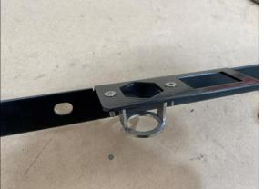
**STEP 2.2** INSTALL JBA-CB101B HOUSING TO SUPPORT BRACKET USING M4 X 16 CSK HEAD SCREW, WASHERS AND NYLOC NUT AS SHOWN.
