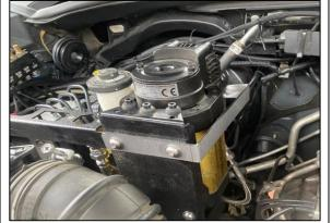
**STEP 3.4** REMOVE THE TWO TOP M8 X 20 DOME HEAD BOLTS AND LOOSLEY INSTALL REAR SUPPORT BRACKET (10-CB255D).
