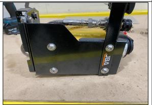
**STEP 1.4** BOLT ON THE OUTLET SUPPORT BRACKET (10-CB255C) FINGER TIGHT (BOLTS NEED TO BE REMOVED LATER)
