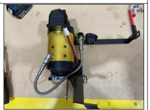
**STEP 2.4** FIT JBA-CB104 0 DEGREE FITTING TO BULK HEAD AND CONNECT 400MM HOSE AS SHOWN.
