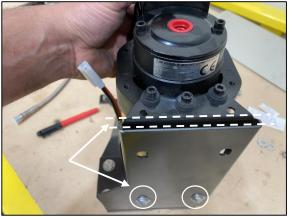
**STEP 1.2** BOLT THE TJM COMPRESSOR TO THE MOUNTING BRACKET IN THE ORIENTATION SHOWN. PUSH THE COMPRESSOR UP SO IT IS JUST ABOVE THE JBA BRACKET AS SHOWN AND FASTEN BOTTOM 2 X BOLTS ONLY.
