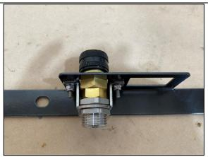
**STEP 2.3** FIT BULK HEAD AND NITTO AS SHOWN. ENSURE LOCTITE IS APPLIED TO THE NUT ON REAR.
