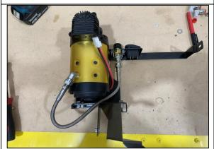
**STEP 1.5** IF INSTALLING JBA-KIT1 AIR/SWITCH OPTION, INSTALL JBA-CB106 90 DEGREE ELBOW AS SHOWN (REFER TO STEPS 2 BELOW FOR FURTHER DETAILED STEPS ON AIR OUTLET).
