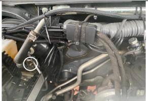
**STEP 3.5** SLIDE THE OTHER END OF THE REAR SUPPORT BRACKET OVER THE M8 STUD ON THE BRAKE BOOSTER AND FASTEN USING M8 WASHER AND NYLOC NUT.
