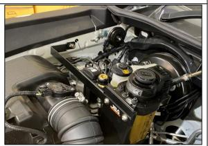
**STEP 3.6** FULLY TIGHTEN ALL FASTENERS AND COMPLETE WIRING AS PER TJM WIRING INSTRUCTIONS. CABLE TIE ANY LOOMS/HOSES NEATLY AND CYCLE/TEST COMPRESSOR AND CONNCETIONS.
