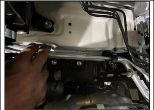
**STEP 3.1** BEND THE AIR CONDITIONER PIPES AWAY FROM THE BODY APPROX 5MM TO ENSURE CLEARANCE FOR NEXT STEP.
