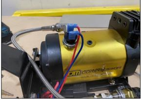
**STEP 1.6** INSTALL TJM PRESSURE SWITCH NEXT TO 90 DEGREE ELBOW.
