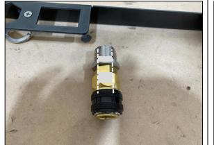
**STEP 2.1** FIT THE TJM NITTO FITTING (NOT SUPPLIED BY JBA) TO THE JBA-CB103 BULKHEAD AND NUT. ENSURE THE FLAT FACES ALIGN AS SHOWN.
