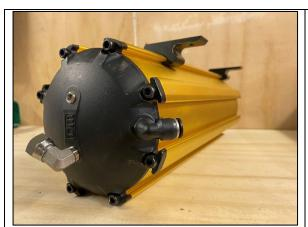
**STEP 1.9** INSTALL JBA 90 DEGREE QUICK FIT ELBOW TO 1/8" PORT AT THE BOOTOM OF THE TANK AS SHOWN.
