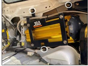
**STEP 2.1** POSITION BRACKET INTO VEHICLE LINING UP THE FACTORY BODY POINTS. INSTALL TOP LEFT AND BOTTOM POSITIONS USING M6 X 20 SEMS SCREW AND TOP RIGHT POINT USING M6 X 20 SEMS WITH M6 FLANGE NUT FROM BEHIND.
