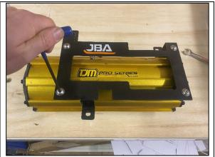
**STEP 1.8** ATTACH THE TANK TO THE JBA BRACKET USING M8 X 20 PAN HEAD WITH A WASHER UNDER THE HEAD AS SHOWN. FASTEN FROM UNDERNEATH USING M8 NYLOC AND WASHER.
