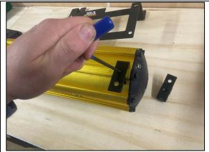
**STEP 1.1** USING A 5MM ALLEN KEY, LOOSEN OFF THE GRUB SCREW ON EACH TANK FOOT AND SLIDE OFF THE TANK.
