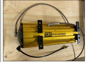
**STEP 1.7** ATTACH JBA STAINLESS HOSES TO ELBOWS PREVIOUSLY INSTALLED IN STEPS 1.5-1.6.
