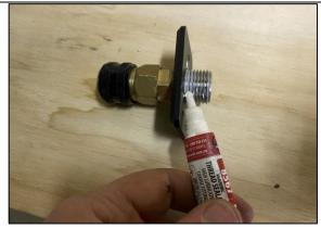
STEP 9 FEED THE BULKHEAD (JBA-CB103) THROUGH THE FRONT OF THE FASCIA (JBA-CB102A) AND APPLY 567 THREAD SEALANT OR LOCTITE AS SHOWN FROM BEHIND.
