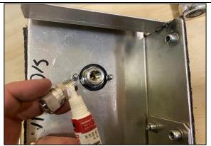
**STEP 12** INSTALL ANY ELBOWS OR HOSES BEING FITTED FROM REAR APPLYING 567 THREAD SEALANT. CLEAN ANY SWARF, CHECK FOR AIR LEAKS AND RE-INSTALL DRAWER FRONT.
