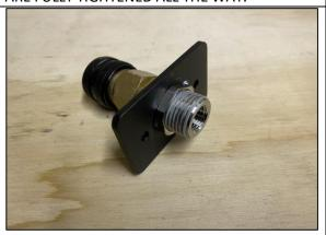
**STEP 10** FASTEN STAINLESS NUT FROM BEHIND AND FULLY TIGHTEN. ENSURE THE FRONT OF THE BULKHEAD IS ALIGNED AND SEATED PROPERLY.
