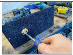
STEP 6 CLEAN CENTRE HOLE DEBURRING ANY SHARP EDGES USING RAT TAIL FILE. COUNTERSINK OUTER 5MM HOLES.
