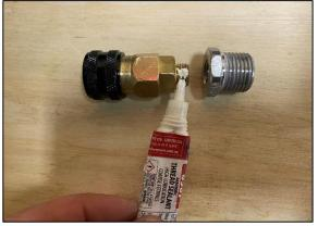
STEP 8 APPLY 567 LOCTITE TO TJM NITTO FITTING (NOT SUPPLIED IN THIS KIT) AND INSTALL TO JBA-CB103 BULK HEAD. THIS WILL BECOME TIGHT TOWARDS THE END AS THE TWO THREADS ARE TAPERED, ENSURE 2 PARTS ARE FULLY TIGHTENED ALL THE WAY.
