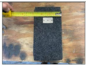
**STEP 1** IDENTIFY THE LOCATION FOR THE AIR OUTLET AND MARK WITH TEXTA/SCRIBE. POSITION THE CENTRE HOLE OF THE DRILLING TEMPLATE OVER PREVIOULSY MARKED POINT.
