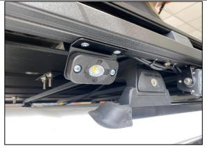
STEP 2- MOUNT THE BRACKET USING M5 X 12 CSK HEAD SCREWS WITH WASHER AND NYLOC NUT FROM REAR.
