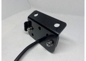
STEP 2.4 FIT ROK9 LIGHT TO JBA BRACKET USING M5 X 16 PAN HEAD AND WASHER WITH NYLOC NUT FROM BEHIND AS SHOWN.
