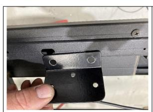
**STEP 1-** SELECT MOUNTING POSITION (NORMALLY EVEN DISTANCE FROM EACH END) NORMALLY ONE HOLE WILL LINE UP WITH A SLOT IN THE RACK. MARK AND DRILL THE OTHER HOLE TO 6MM.
