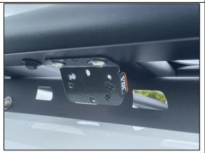
STEP 3.3- FIT BRACKET TO RACK USING M8 BUTTON HEAD WITH SPRING WASHER ON UNDER SIDE AND M8 WASHER WITH NYLOC NUT FROM TOP SIDE (ON ALL HOLES NOT UTILISING CHENNEL NUT AS PER STEP 3.1, OPTION 1).
