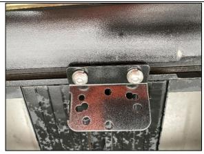
**STEP 2.3** SLIDE THE BRACKET ALL THE WAY INTO THE CHANNEL AND TIGHTEN FULLY WHEN IN POSITION.
