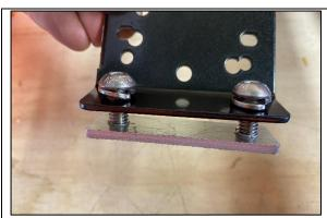
**STEP 2.1** FIT THE NUT PLATE TO THE JBA BRACKET USING M8 BUTTON HEAD WITH SPRING WASHER AS SHOWN. ONLY SCREW IN TO NUT PLATE 1-2 TURNS.
