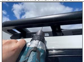
**STEP 3.2**- DRILL OUT MARKED HOLES TO 8-9MM. IT IS EASIE TO DO THIS WITH THE RACK OFF THE VEHICLE IF POSSIBLE.
