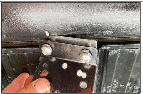
**STEP 2.2** SLIDE ONE END OF THE NUT PLATE INTO THE CENTRE OPENING OF THE REAR CHANNEL OF THE RACK
