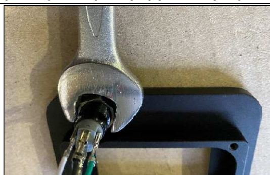
STEP 1.2.4 INSERT SWITCH IN TO FASCIA AND TIGHTEN NUT FROM REAR USING 14MM SPANNER.
