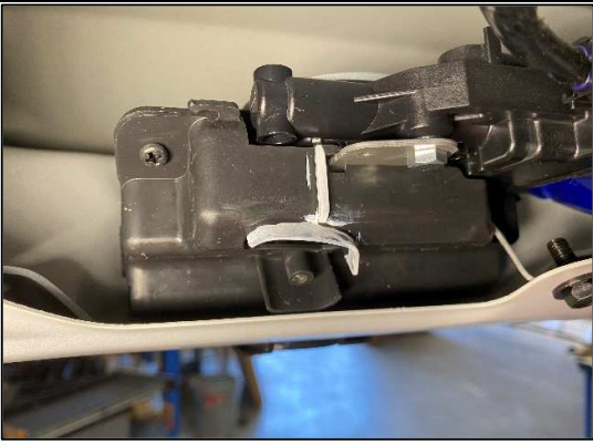
STEP 1.1.2 THE SECTIONS OUTLINED IN WHITE NEED TO BE REMOVED, NOTE AND MARK THE AREAS SHOWN.
