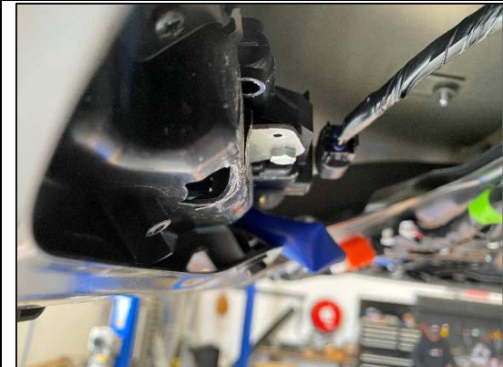
STEP 1.1.3 TRIM BACK THE RAISED SECTIONS MARKED IN PREVIOUS STEP SO THEY ARE COMPLETELY FLAT AS SHOWN.
