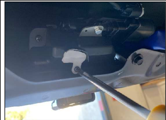
STEP 1.1.1 REMOVE THE WHITE PLASTIC COVER ON THE AUTO LOCKING LOCK AS SHOWN.
