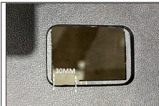
STEP 1.2.1 NOTCH OUT THE BOTTOM LIP OF THE INSERT SECTION 30MM AS SHOWN
