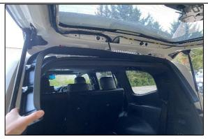
STEP 3.1 REMOVE THE REMAINING TAILGATE SECTIONS (FROM STEPS 1.1-1.5) ON BOTH SIDES AND ALONG THE TOP. WHEN REMOVING THE SIDE SECTIONS ON THE TAILGATE, CHECK FOR BODY CLIPS REMAINING IN THE VEHICLE.
