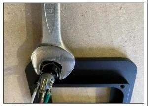
STEP 2.5 OPTIONAL STEP- ONLY COMPLETE IF FITTING JBA SWITCH TO FASCIA. INSERT SWITCH IN TO FASCIA AND TIGHTEN NUT FROM REAR USING 14MM SPANNER.
