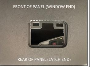
**STEP 1.6** REMOVE THE REAR SECTION AND PLACE ON A SOFT CLEAN SURFACE. MARK THE INFILL SECTION AS SHOWN.
