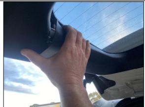
**STEP 1.5** SEPARATE THE MID SECTION FROM THE REAR SECTION AS SHOWN TO ENABLE ACCESS TO THE REMAINDER OF THE TRIM CLIPS IN THE REAR SECTION.
