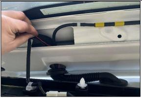
**STEP 3.4** FEED THE WIRE THROUGH THE GROMMET AND INTO THE TAILGATE SECTION AS SHOWN.
