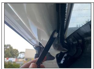
**STEP 1.9** REFERENCE PICS FOR TRIM CLIPS (EXAMPLE ONLY). AS YOU ARE REMOVING PANELS, KEEP NOTICE OF ANY CLIPS THAT HAVE REMAINED IN THE VEHICLE AND REMOVE WITH TRIM CLIP REMOVER.
