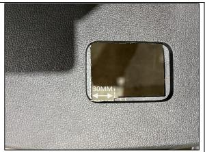
**STEP 1.8** ONLY COMPLETE THIS STEP IF FITTING OPTIONAL SWITCH TO FASCIA. TRIM BOTTOM LEFT SECTION APPROX 30MM AS SHOWN ON THE REAR OF THE PANEL SIDE.
