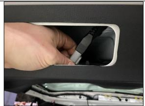
**STEP 4.1** RE-INSTALL REAR TAILGATE PANELS AND PLUG LED LIGHT INTO WIRING INSTALLED IN STEPS 3.1 TO 3.5 ABOVE.
