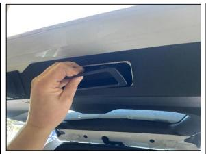
**STEP 1.1** REMOVE 2 X REAR HANDLE INSERTS PULLING DOWN FROM THE TOP CENTRE AND LEVERING FORWARD.
