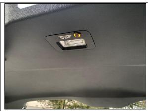
**STEP 4.2** TEST LED LIGHT AND WIPE DOWN PANELS.
