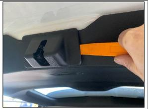
**STEP 1.2** USING A PLASTIC TRIM TOOL, LEVER THE CENTRE LATCH COVER AND REMOVE.
