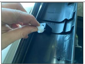
**STEP 1.10** RE-INSERT CLIPS INTO THE PLASTIC TRIM PANEL LOCATION. THEY WILL NORMALLY SLIDE IN AND POP INTO POSITION. THIS STEP WILL ENSURE AN EASIER RE-INSTALLATION OF THE PANELS LATER.
