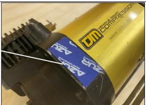
**STEP 2.2** APPLY ANTO VIBRATION TAPE TO THE MOTOR END ON THE INSIDE FACE AS SHOWN.
