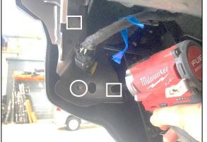
**STEP 1.9** IN BEHIND THE FLARE, REMOVE TORQ SCREW AS SHOWN.
