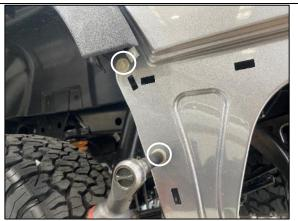
**STEP 1.14** REMOVE 2 X M6 SCREWS ON OUTSIDE OF BODY.
