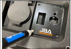
**STEP 3.1.1** REMOVE 12V PANEL FROM VEHCILE AND PLACE ON WORK BENCH. PLACE FASCIA PLATE IN RHS GAP AND MARK OUTER SCREW HOLES AS SHOWN.
