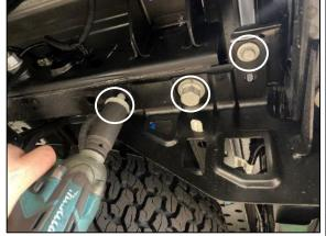
**STEP 1.1 IF NO TOWBAR FITTED** REMOVE REAR BUMPER BY REMOVING 3 X BOLTS SHOWN EACH SIDE.
