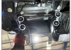
**STEP 1.13** REMOVE 4 X M10 BOLTS STEP FRAME. NOTE- THESE HAVE LOCTITE APPLIED FROM FACTORY AND TAKE SOME CONVINCING.
