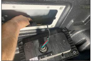
STEP 4.4 FROM INSIDE THE TUB, SHAKE THE COMPRESSOR AND CHECK THAT THAT THERE IS NO MOVEMENT BETWEEN THE COMPRESSOR AND TUB BODY. IF THERE IS ANY MOVEMENT, LOOSEN BRACKET AND RE-ADJUST. THIS STEP IS CRITICAL AND WILL ENSURE THAT THE COMPRESSOR WILL NOT BOUNCE WHILE DRIVING AND CAUSE DAMAGE TO THE OUTER BODY PANEL.
