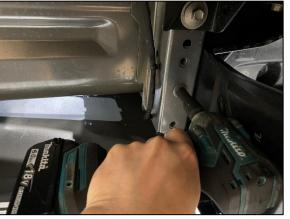
**STEP 1.18** REMOVE M6 SCREW AND KEEP ASIDE FOR BRACKET INSTALLATION.
