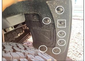
**STEP 1.7** REMOVE 6 X PLASTIC CLIPS (CIRCLES) AND 1 X TORQ SCREW (SQUARE) AS SHOWN. TO REMOVE PLASTIC CLIPS, UNSCREW WITHOUT PUSHING ON THE SCREW GENTLY.
