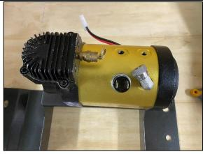
**STEP 2.3** FIT JBA-CB106 90 DEGREE ELBOW TO BOTTOM RIGHT 1/4" GRUB SCREW AND FACE 45 DEGREES TO THE LEFT AS SHOWN. INSTALL TJM PRESSURE SWITCH ON THE BOTTOM LEFT 1/8" SCREW. CONNECT RELEVANT HOSE FROM KIT BEING USED- 400MM FOR KIT 2 AND 1200MM FOR KIT 4.
