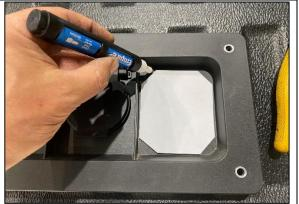
**STEP 3.1.2** MARK OUT CUTTING TEMPLATE AROUND SCREW LOCATIONS MARKED IN PREVIOUS STEP.
