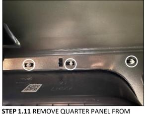
**STEP 1.11** REMOVE QUARTER PANEL FROM VEHICLE WORKING ALONG PUSHING THROUGH THE PLASTIC CLIPS. **TIP**- AN 8MM SOCKET CAN BE USED TO SQUEEZE THE CLIP.
