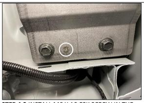
**STEP 4.2** INSTALL M6 X 16 CSK SCREW IN THE HOLE AT THE REAR OF THE VEHICLE WITH WASHER AND WHIZZ NUT FROM ABOVE (NOT FULLY TIGHTENED)
