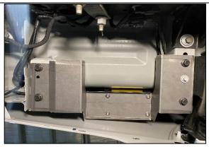
**STEP 4.1** LIFT COMPRESSOR AND BRACKET INTO PLACE AND INSTALL 4 X M10 BOLTS AND 1 X M6 BOLTS REMOVED IN STEP 1.13 AND 1.16 ABOVE **(DON'T TIGHTEN FULLY YET)**
