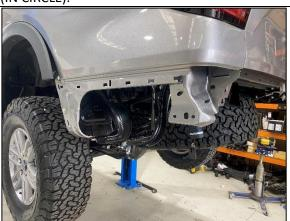
**STEP 1.12** FULLY REMOVE REAR PANEL AS SHOWN AND SET ASIDE.
