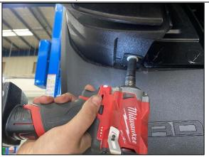
**STEP 1.6** REMOVE MUDFLAP, START BY REMOVING M6 SCREW FROM UNDERNEATH AS SHOWN.
