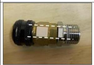
**STEP 3.1.4** FIT JBA-CB101B HOUSING TO FASCIA PLATE USING M4 X 16 CSK SCREWS. ASSEMBLE JBA-CB103 BULKHEAD WITH NITTO AS SHOWN ENSURING FLAT FACES ARE IN LINE. INSTALL ASSEMBLY INTO FASCIA AND FASTEN NUT FROM BEHIND- ENSURE LOCTITE APPLIED TO NUT
