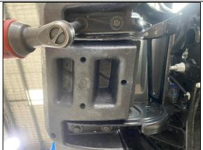
**STEP 1.5** REMOVE PLASTIC STEP BY REMOVING 4 X M6 SCREWS FROM UNDERSIDE. SET ASIDE FOR REFITMENT LATER.
