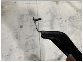
**STEP 1.17** ONCE REMOVED, BEND TAB WITH THE PIN UP SLIGHTLY AS SHOWN.
