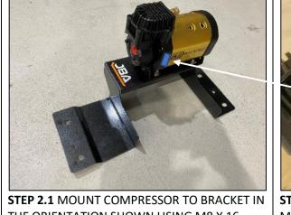
THE ORIENTATION SHOWN USING M8 X 16 DOME HEADS WITH WASHER UNDER THE HEAD FROM UNDERNEATH THE BRACKET AND M8 NYLOC NUT WITH WASHER FROM COMPRESSOR SIDE.
