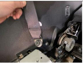
**STEP 1.10** REMOVE PASSENGER SIDE REAR SEAT BELT USING 14MM SOCKET.
