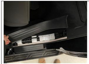
**STEP 1.1** START AT THE REAR PASSENGER SIDE DOOR, FOLD THE PASSENGER SECOND ROW OF SEATS FORWARD AND REMOVE PLASTIC TRIM LEVERING UP FROM BODY CLIPS AS SHOWN.
