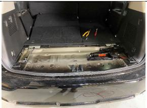
**STEP 1.6** STARTING FROM THE LEFT OR RIGHT SIDE, PULL UP THE REAR PLASTIC TRIM AND WORK ACROSS TO FULLY REMOVE. CHECK FOR ANY TRIM CLIPS.
