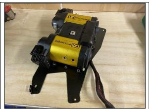
**STEP 2.1**. MOUNT THE TWIN TJM COMPRESSOR IN THE ORIENTATION SHOWN. USE M8 X 16 SCREW WITH A WASHER UNDER THE HEAD AND M8 NYLOC NUT WITH WASHER FROM BEHIND.
