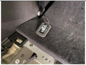
**STEP 1.7** REMOVE 2 X TIE DOWN POINTS USING 10MM SOCKET. IT IS EASIER TO POP THE PLASTIC INNER COVER THROUGH THE TIEDOWN AS SHOWN TO ACCESS THE BOLT.
