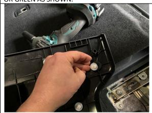
**STEP 1.20** RE-INSERT INTO THE PLASTIC TRIM PANEL LOCATION. THEY WILL NORMALLY SLIDE IN AND POP INTO POSITION. THESE STEPS WILL ENSURE AN EASIER RE-INSTALLATION OF THE PANELS LATER.
