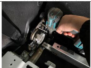
**STEP 1.9** REMOVE BOLTS FROM PASSENGER SIDE REAR SEAT USING 14MM SOCKET AND PULL SEAT OUT.
