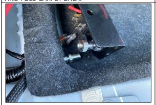
**STEP 4.1.5** FEED THE AIRLINE, SWITCH LOOM AND FUSE WIRES THROUGH THE HOLE JUST CUT IN STEP 4.4.
