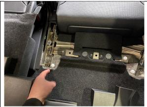
**STEP 1.18** REFERENCE PICS FOR TRIM CLIP (EXAMPLE ONLY). AS YOU ARE REMOVING PANELS, KEEP NOTICE OF ANY CLIPS THAT HAVE REMAINED IN THE VEHICLE- NORMALLY WHITE OR GREEN AS SHOWN.
