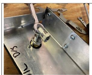
**STEP 4.2.1** PREPARE DRAWER FRONT OUTLET FOLLOWING JBA-CB101 INSTRUCTIONS. INSTALL JBA-CB106 90 DEGREE ELBOW TO REAR OF DRAWER FRONT AND TIGHTEN FACING DOWN (BOTTOM OF DRAWER FRONT). CONNECT 400MM HOSE.
