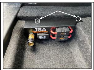
**STEP 4.1.7** FEED THE POWER WIRE THROUGH EITHER SIDE OF THE FUSE, TERMINATE AND HEAT SHRINK. INSTALL THE BRACKET TO THE BODY PLUGS EXPOSED IN STEP 4.3 USING 14G X 1 CSK PHIL SELF TAPPER.
