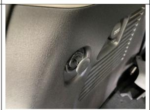
**STEP 1.12** REMOVE REAR TRIM CLIP NEXT TO 12V SOCKET AS SHOWN.
