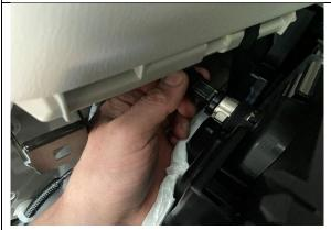
STEP 1.17 THE QUARTER PANEL SHOULD BE FREE NOW. UNPLUG THE 12V SOCKET FROM THE REAR AND CAREFULLY REMOVE THE QUARTER PANEL FROM THE VEHICLE. CHECK FOR ANY TRIM CLIPS IN THE BODY (REFER TO STEPS 1.18-1.20 BELOW)
