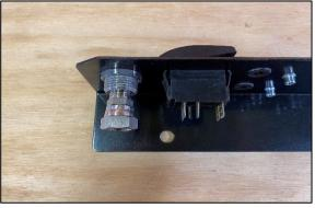
STEP 4.1.2 FIT JBA-CB104 0 DEGREE ELBOW USING 567 THREAD SEALENT ON THE REAR OF THE BULKEAD. INSTALL TJM NITTO FITTING (SUPPLIED IN 013COMPAKN) USING 567 THREAD SEALANT TO FRONT OF BULK HEAD.
