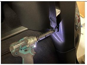
**STEP 1.2** REMOVE THE SECOND ROW SEAT BELT USING 14MM SOCKET.
