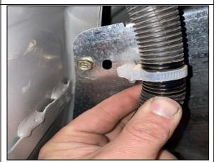
**STEP 3.6** RECLIP THE MAIN BODY LOOM REMOVED IN STEP 3.4 INTO THE COMPRESSOR BRACKET ON THE LEFT HAND SIDE SLOTS ALLOCATED.
