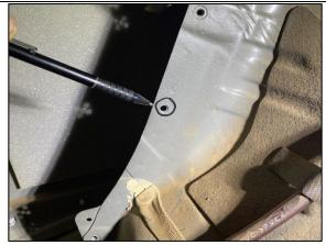
**STEP 3.3**. LOCATE THE BODY HOLE JUST ABOVE THE BODY SEAL TRIMMED IN STEP 3.2 AND CLEAR OUT TO 7MM. TREAT WITH RUST SEALANT.
