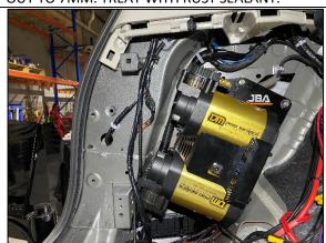
**STEP 3.5** LIFT THE COMPRESSOR BRACKET INTO PLACE AND FASTEN INTO BODY CAPTIVE NUTS USING M6 X 20 SEMS FASTENERS. USE M6 WHIZZ NUT FROM BEHIND THE 7MM HOLE CLEARED IN STEP 3.3 ABOVE .
