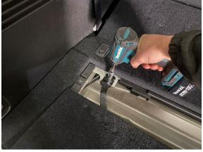
**STEP 1.4** REMOVE 2 X M6 BOLTS USING 10MM SOCKET AND REMOVE REAR INFILL FROM VEHICLE.
