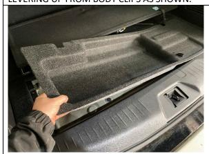
**STEP 1.3** MOVE TO REAR OF THE VEHICLE AND REMOVE REAR STORAGE INSERT.
