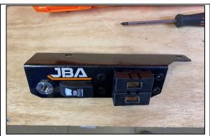
**STEP 4.1.1** INSTALL CARLING SWITCH AND ANSH FUSE HOLDERS (SUPPLIED WITH TJM COMPRESSOR) USING M4 X 12 SCREWS. INSTALL JBA-CB103 BULK HEAD AS SHOWN, APPLY THREAD SEALANT TO NUT FROM BEHIND.
