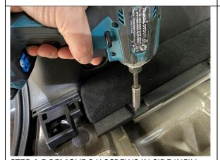
**STEP 1.5** REMOVE 2 X SCREWS IN SIDE INFILL SECTION USING 10MM SOCKET AND REMOVE. CHECK FOR TRIM CLIPS.
