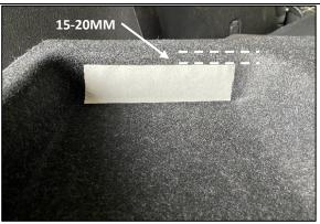
**STEP 4.1.4** CUT A HOLE OUT OF THE END OF THE CARPET APPROX 15-20MM FROM ALL EDGES AS SHOWN
