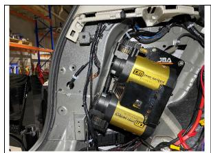
**STEP 5.1** NEATLY CABLE TIE AND LOOSE LOOMS AND AIR LINES. TEST ALL AIR CONNECTIONS FOR AIR LEAKS AND CYCLE COMPRESSOR CHECKING ELECTRICAL FUNCTIONALITY.
