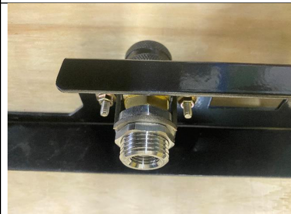
STEP 3.1.3 INSTALL ASSEMBLY INTO FASCIA AND FASTEN NUT FROM BEHIND- ENSURE LOCTITE APPLIED TO NUT.
