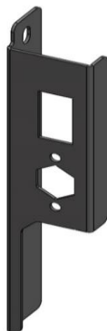
STEP 3.1.5 INSTALL INTO VEHICLE USING M8 X 20MM. FOR VEHICLES WITH LINER PLACE 10MM SPACER BEHIND BRACKET ON TOP HOLE.
