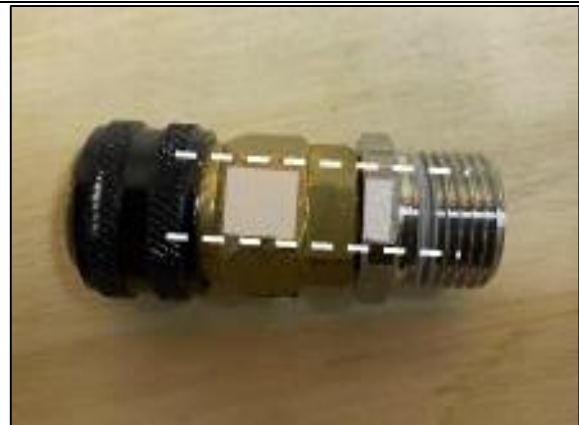
STEP 3.1.2 FIT JBA-CB101B HOUSING TO FASCIA PLATE USING M4 X 16 CSK SCREWS. ASSEMBLE JBA-CB103 BULKHEAD WITH NITTO AS SHOWN ENSURING FLAT FACES ARE IN LINE.
