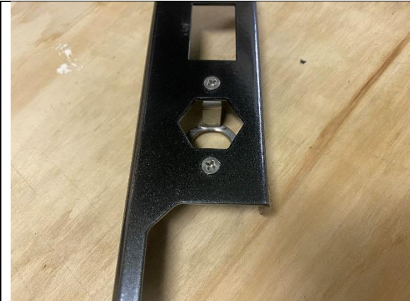
STEP 3.1.1 INSTALL JBA-CB101B COMPRESSOR HOUSING BRACKET USING M4 X 16 CSK SCREWS, WASHERS AND NYLOC NUT.
