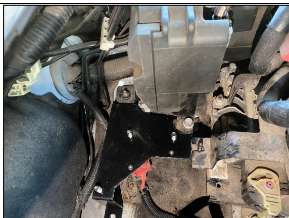
STEP 1.9 SLIDE JBA-CB251SE-A BASE BRACKET INTO THE ENGINE BAY AS SHOWN AND RE-INSTALL 2 X M8 SCREWS REMOVED PREVIOUSLY.
