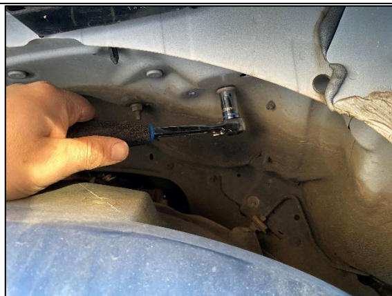
STEP 1.8 REMOVE REAR M8 BOLT FROM UNDERSIDE IN WHEEL ARCH USING 13MM SOCKET AS SHOWN.
