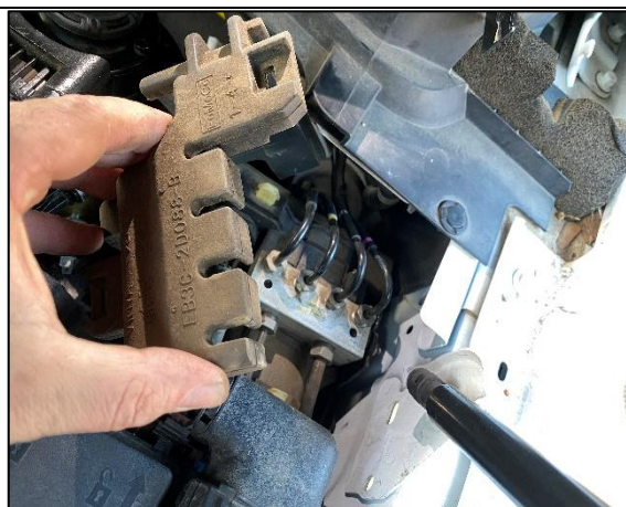
STEP 1.12 IF FITTED, REMOVE THE TOP COVER AS SHOWN PUSHING IN EITHER SIDE OF THE 2 TABS.
